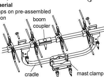
For vertical polarisation rotate cradle through  $90^\circ$  in mast clamp.
